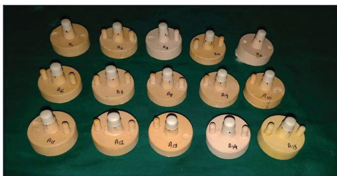
[Table/Fig-4]: Zirconia copings-Group A test samples.
