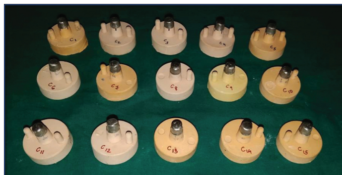
[Table/Fig-6]: CAD/CAM cobalt chromium copings - Group C test samples.
