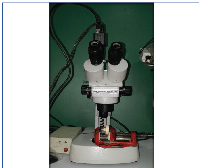
[Table/Fig-8]: Stereomicroscope (Wuzhou New Found Instrument Co. Ltd., China, Model: Xtl 3400e).
