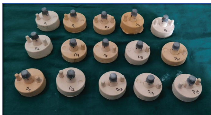
[Table/Fig-7]: Direct metal laser sintered copings - Group D test samples.
